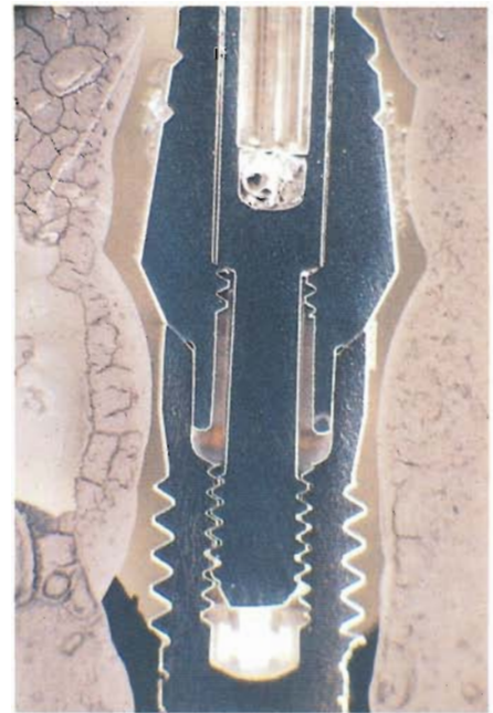
Figure 6—Optical cross-sectional micrographs of each of the Screw-Vent 95 implant/abutment pillars were evaluated. This illustrates the characteristic intimate contact and frictional fit between the internal straight hexagon of the implant and the external 1-degree tapered external hexagon of the abutment. The implant/abutment beveled seating surface also demonstrates full contact and intimate seal. Note the crisp, sharp, internal threads in the implant and corresponding full engagement of the abutment screw threads.
