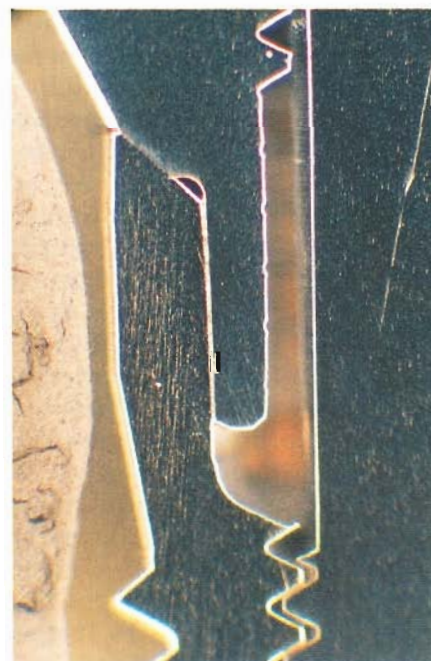
Figure 7—Higher magnification optical micrograph illustrating the friction/interference fit along the entire length of the internal and external tapered hexagonal flats. The 45-degree beveled implant/abutment seating surfaces contact intimately without any discernible interface gap.
