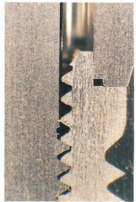
Figure 13—Higher magnification of the hexagonal engagement and the implant/abutment interface, demonstrating excellent intimate contact.
